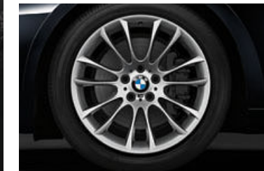
■ 19" M light alloy wheels V-spoke 302 M with mixed tyres. Front: 8.5 J x 19 with 245/45 R 19 tyres. Rear: 9.5 J x 19 with 275/40 R 19 tyres.
