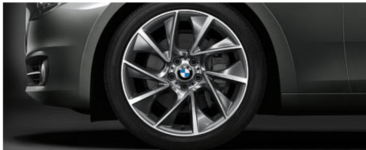
□ 20" light alloy wheels Turbine Styling 457 in Bicolour Ferric Grey with mixed tyres. Front: 8.5 J x 20 with 245/40 R 20 tyres. Rear: 10 J x 20 with 275/35 R 20 tyres.
